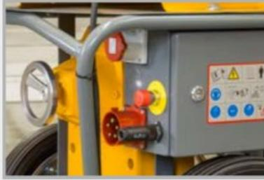
Central control cabinet is also a power distributor for attached devices such as a pan mixer or compressors
