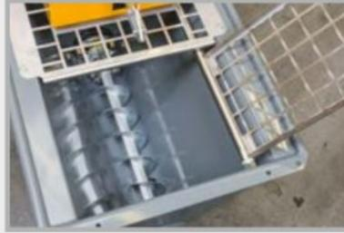
Safety grill with integrated safety switch and wide opening angle provides full access for maintenance and cleaning
